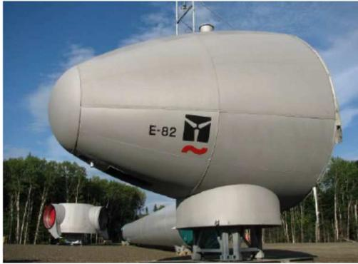
ENERCON E-82 2 MW Direct Drive Wind Turbine nacelle prior to being craned onto 98m tower
